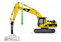
Hammer Work. The front parts automatically follow the hammer while penetrating the rock. Blank shots or excessive force on the hammer are avoided resulting in longer life for the hammer and the machine. Similar advantages with vibratory plates.
