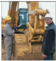
**Bucket Linkage**. Two bucket linkages (B1 and CB2) are available, with lifting eye on the power link.
