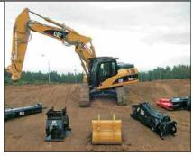
**Work Tools.** Choose from a variety of work tools such as hammers, crushers, pulverizers, shears, multiprocessors and grapples.
