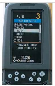
Electronic Control System. Ten hydraulic pump flow and pressure settings can be preset, eliminating the need to adjust the hydraulics each time a tool is changed.
